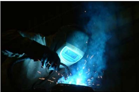
*Flux-Cored Arc Welding (FCAW)*
