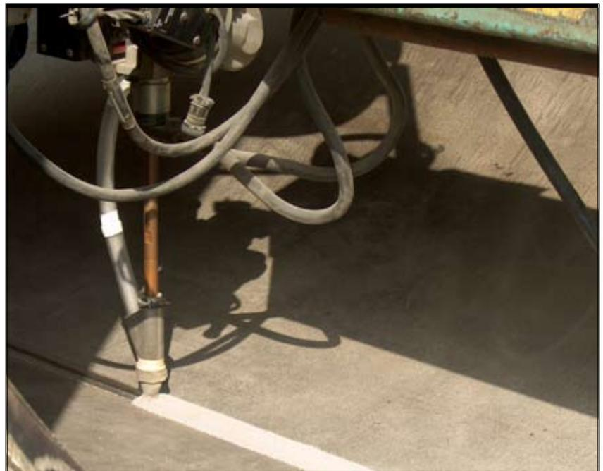
*Submerged Arc Welding (SAW)*
