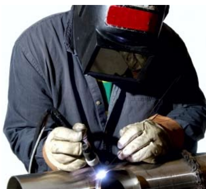
Gas Tungsten Arc Welding
